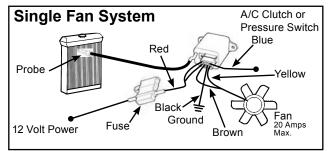
**Dual Fan Systems:** Attach **Brown Wire** to one fan and **Yellow Wire** to other fan motor. This System will handle 2 fans drawing up to 10 Amps each for a total load of 20 Amps. Finish wiring system per the illustration.
