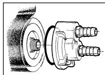
2. Install hose fittings in the engine adapter ports. Seal the threads with Teflon® tape or appropriate sealer on tapered fittings.
