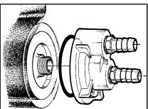
2. Install hose fittings in the engine adapter ports. Seal the threads with Teflon® tape or appropriate sealer on tapered fittings.
