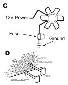
ALLOW PULLTAB TO BE SUPPORTED BY COOLING FIN NOT TUBE
